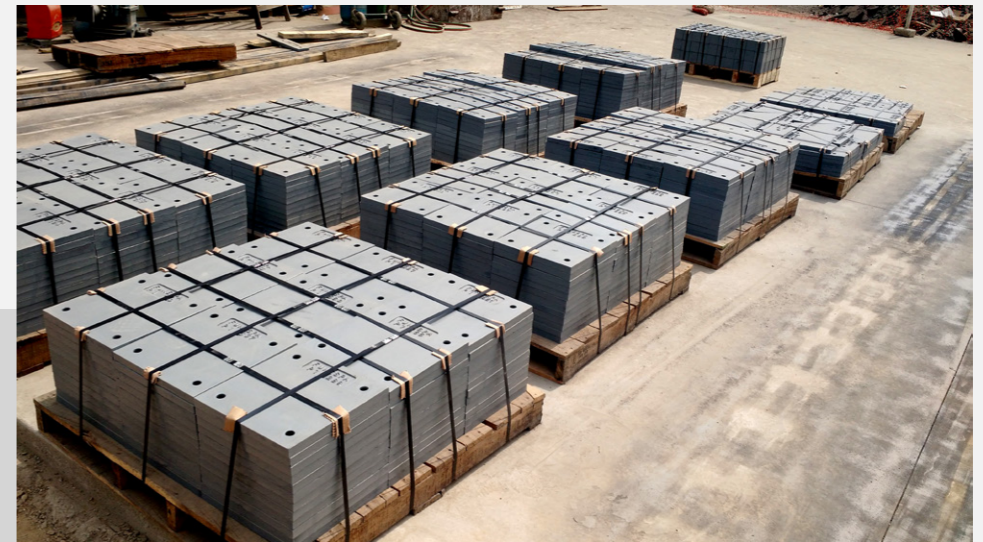
LINERS FOR PREHEATER
